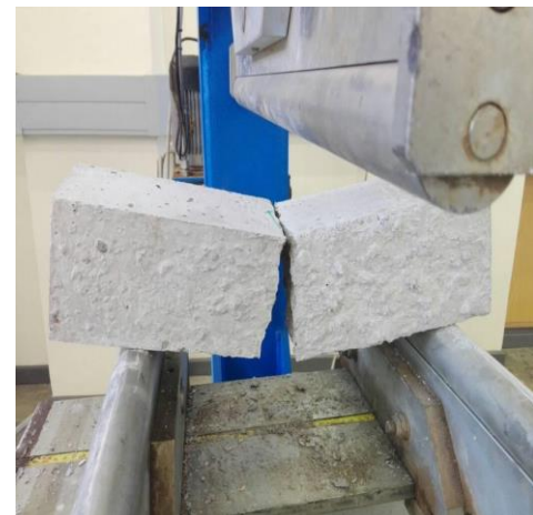
Figure 3 Scheme of flexure test machine in this study
