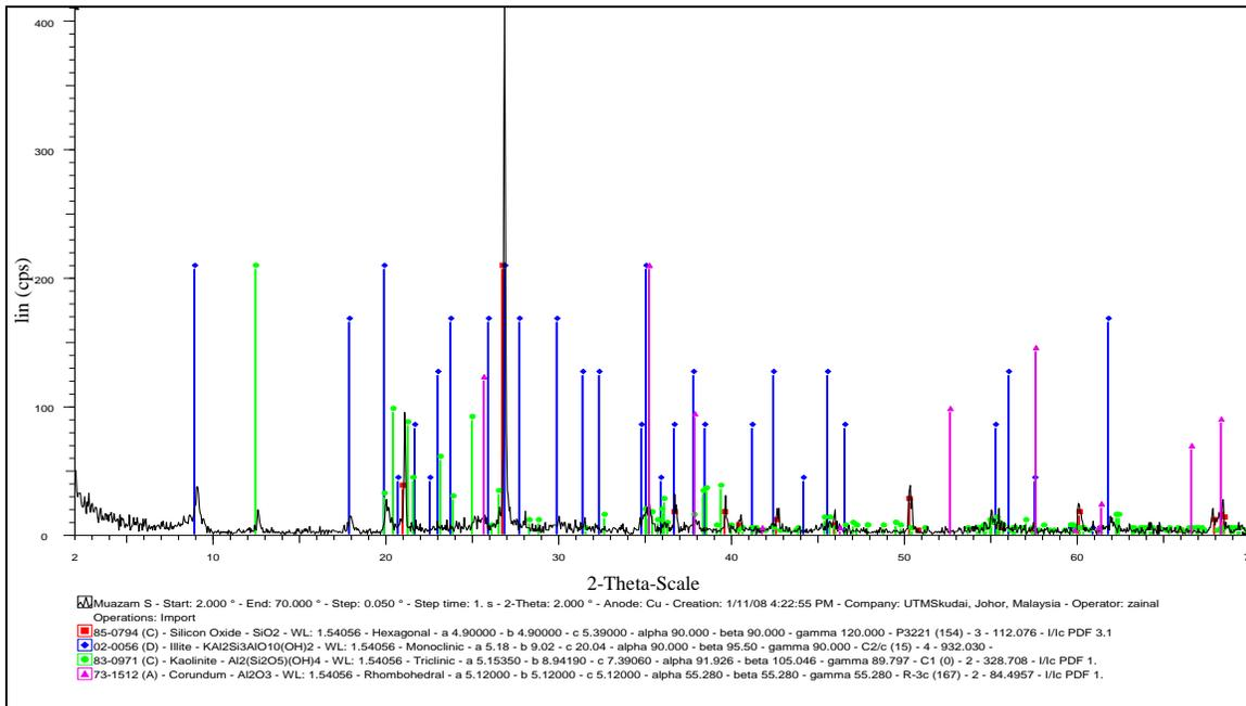
Figure 2 Minerals analysis for the shale sample from Muadzam Shah
