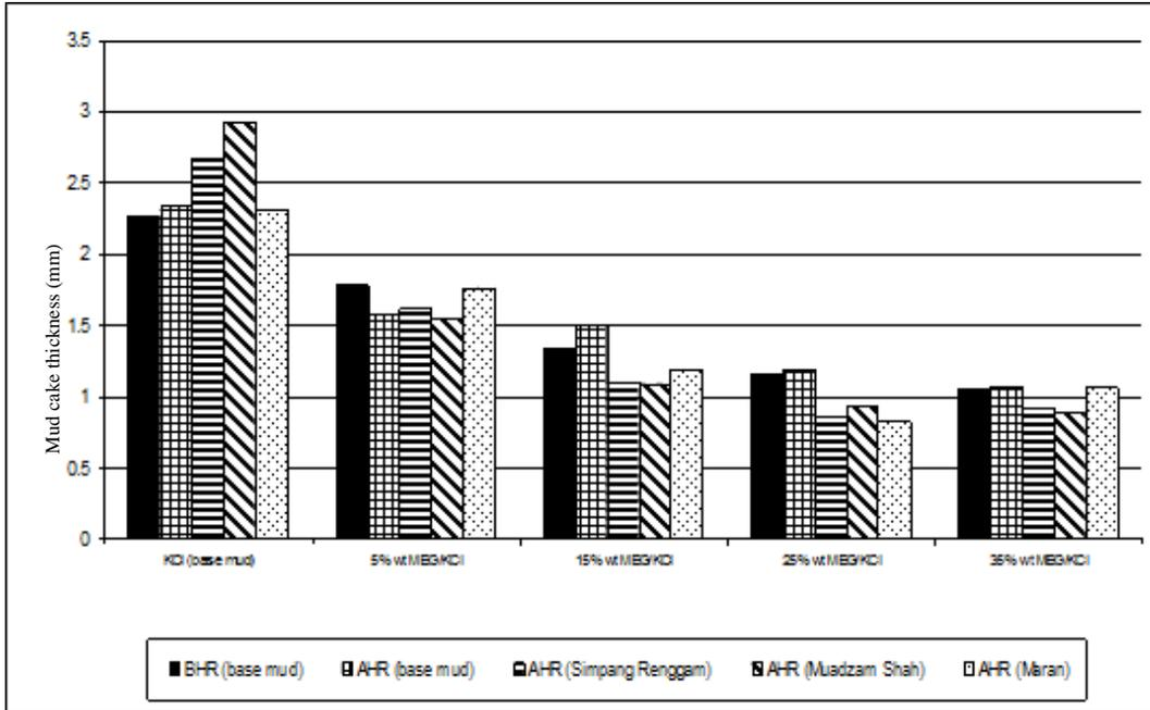
**Figure 10** Mud cake thickness of various drilling mud samples
