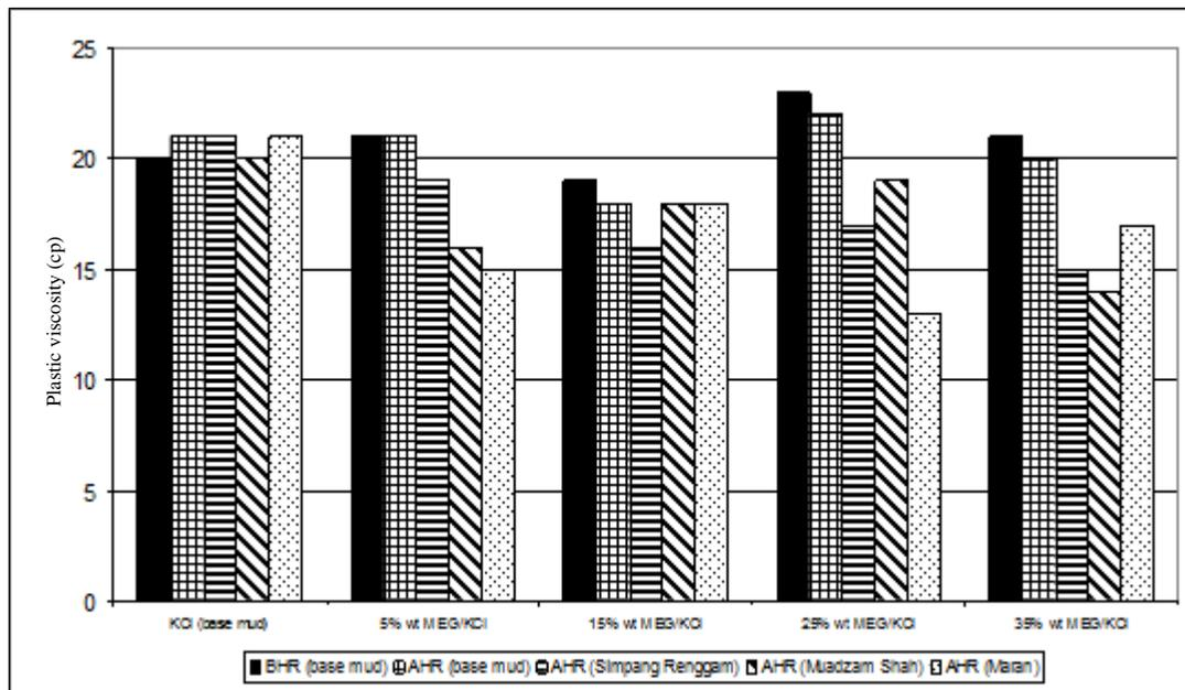
Figure 5 Plastic viscosities of various drilling mud samples
