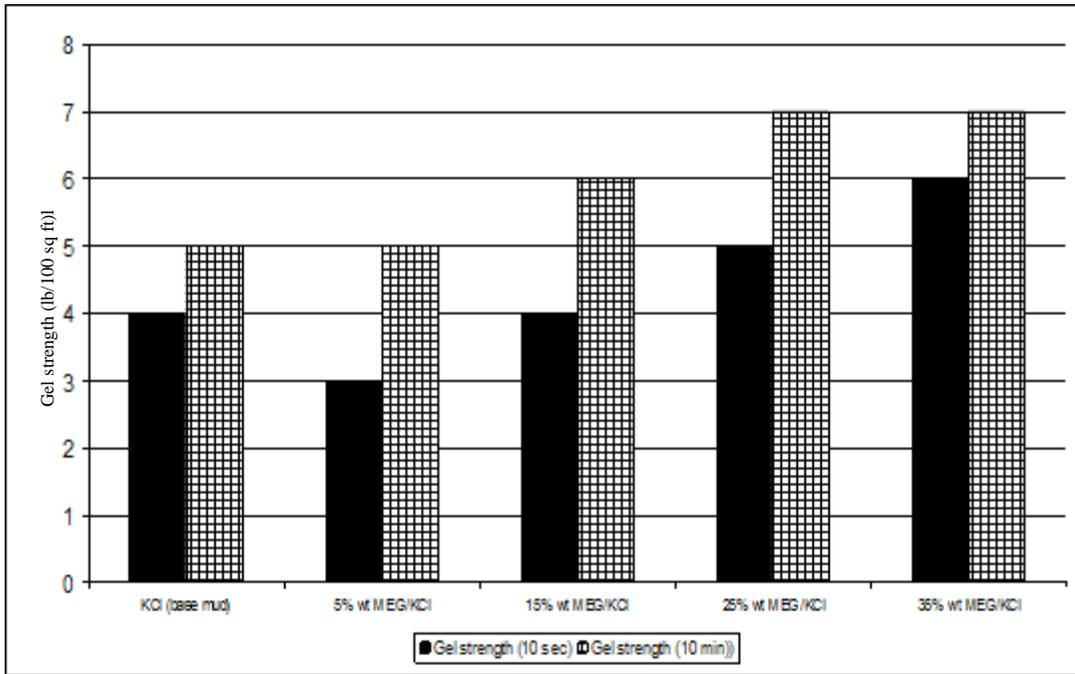
**Figure 8** Gel strength of various drilling mud samples after hot rolling
