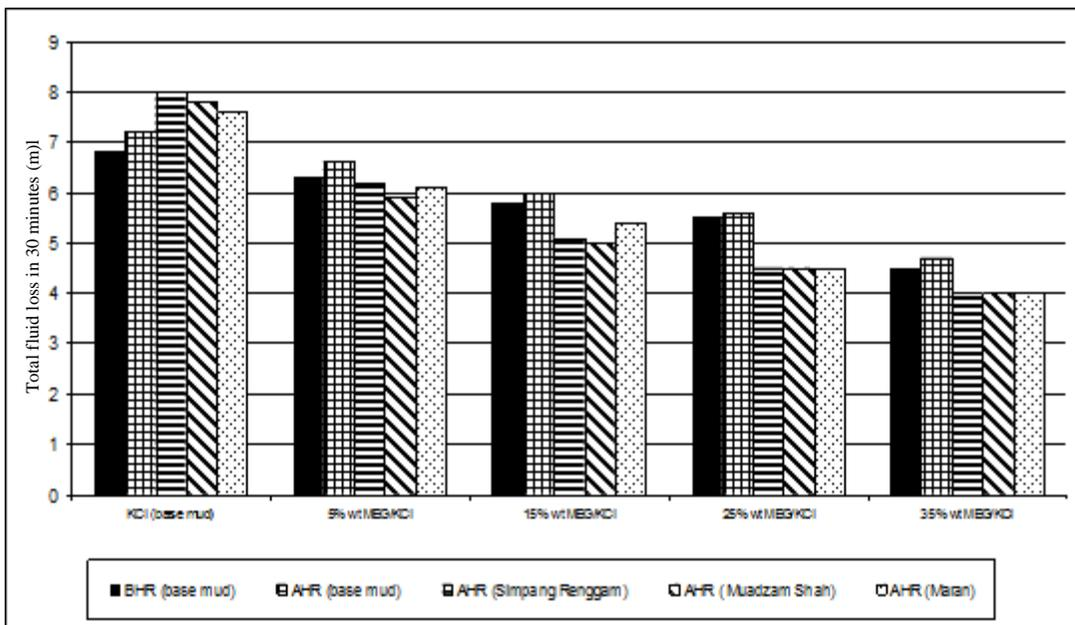
**Figure 9** Total 30 min fluid loss of various drilling mud samples
