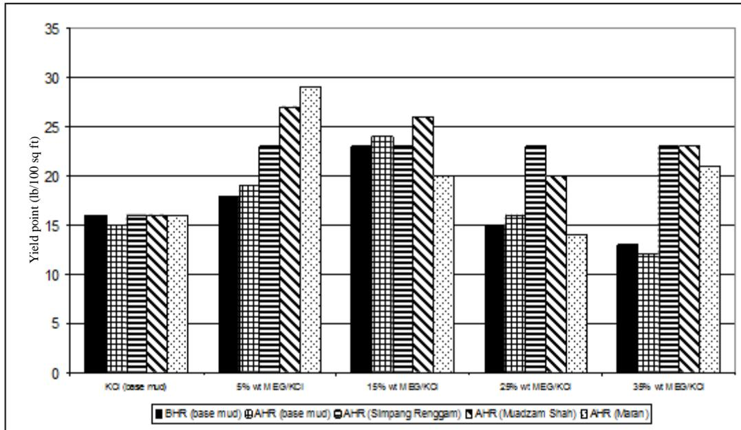
**Figure 6** Yield point of various drilling mud samples
