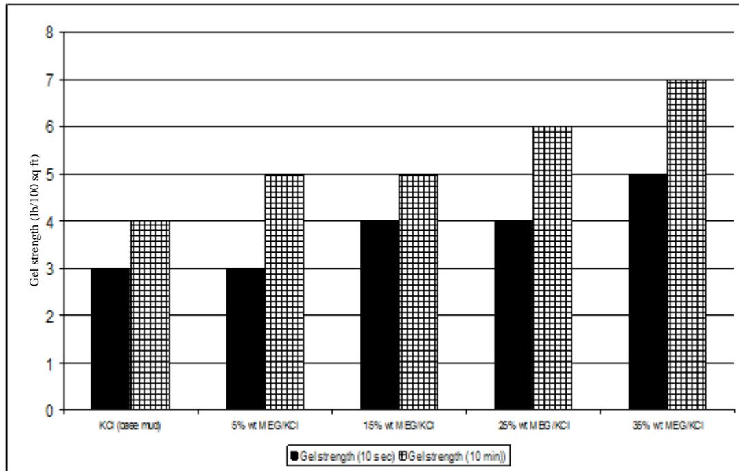
**Figure 7** Gel strength of various drilling mud samples before hot rolling
