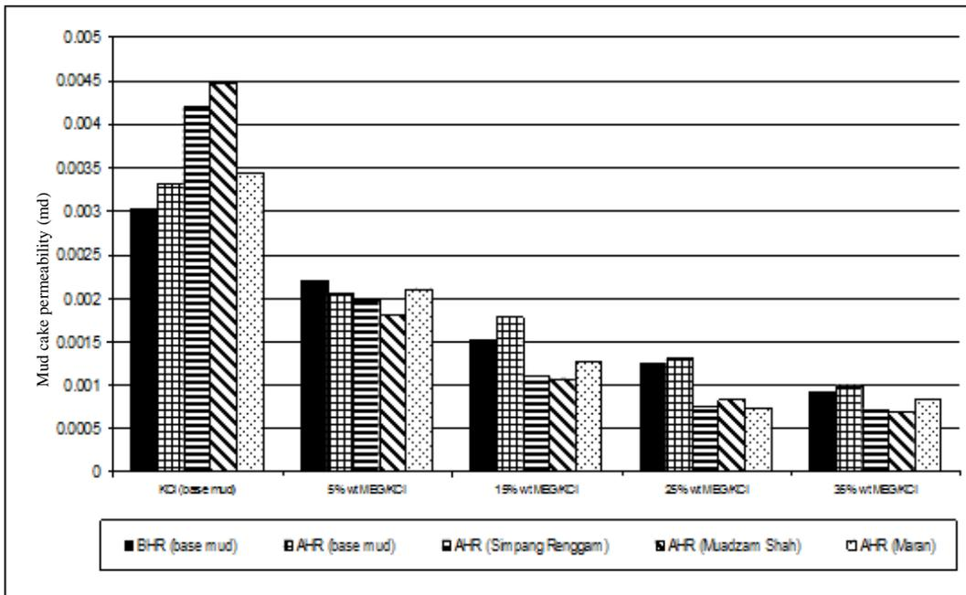
**Figure 11** Mud cake permeability of various drilling mud samples
