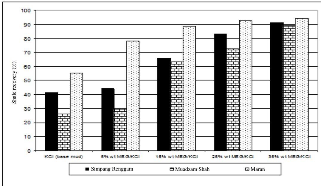
Figure 4 Shale recovery after 16 hours hot rolling dispersion test at 180°F
