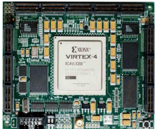
Figure 7 FPGA as channel simulator
