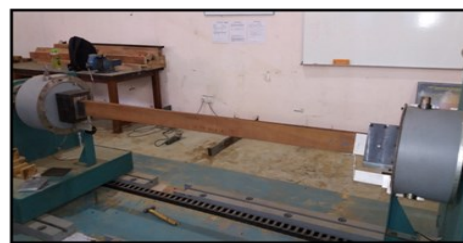
Figure 2 The actual equipment and test set-up for torsion test
