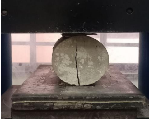
Figure 3 Cylindrical specimen tested in tensile splitting test machine
