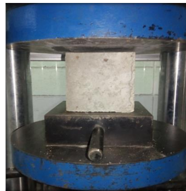
Figure 2 Cube specimen inside compression test machine
