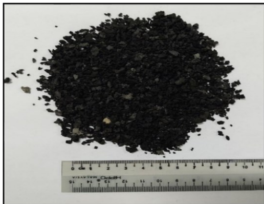
Figure 3 Crumb rubber as sand replacement
