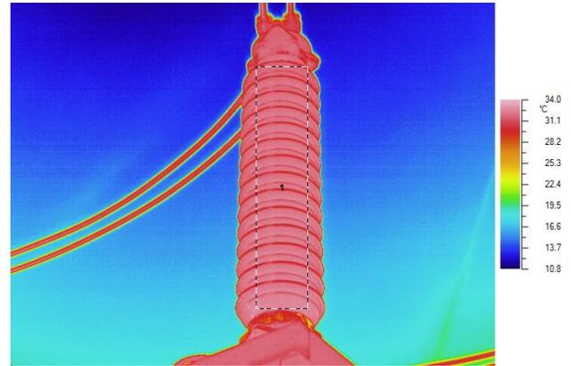
Figure 6 Thermal image 132 kV arrester
