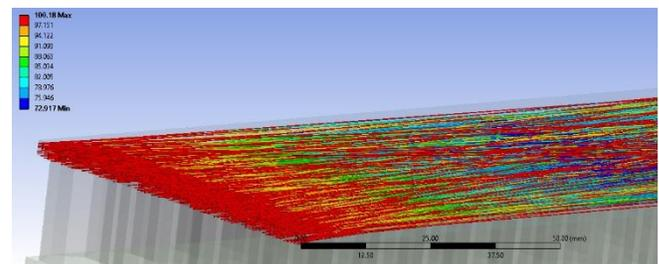
**Figure 10** Temperature distribution on 600 fibers of palm oil
