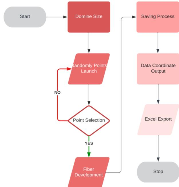
**Figure 4** Fiber development flow by using MATLAB software
