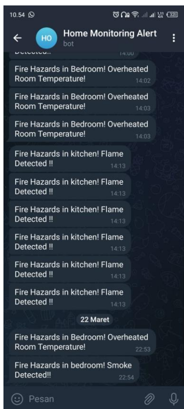
Figure 17 Telegram notification for fire mitigation
