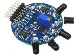
(c) Flame and gas sensor - 5 channel Images Source: https://components101.com
