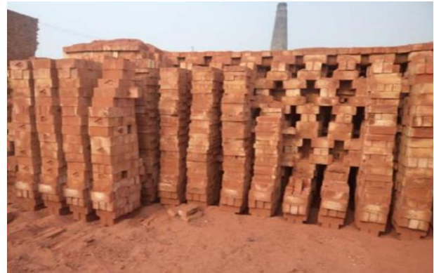
Figure 1 Burnt brick from kiln
