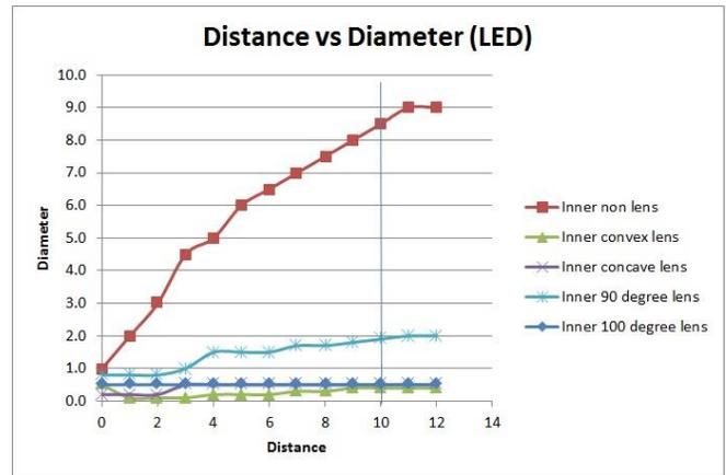
Figure 3.2 Result for inner circle for inner LED
