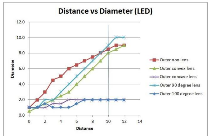
Figure 3.3 Result for outer circle with LED – concave 0.5
