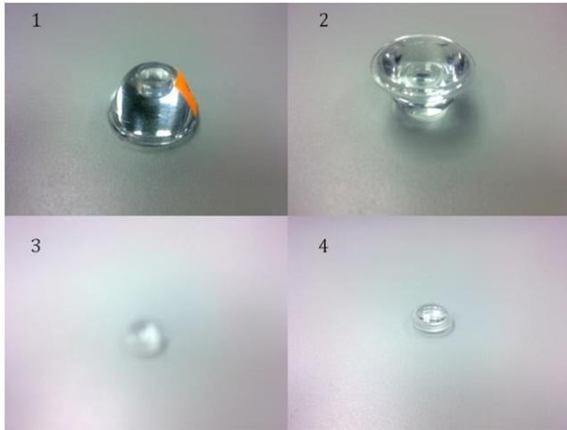
**Figure 1.5** The lenses used in this test:- (1) 90° convex lens;. (2) 100° convex lens;. (3) concave lens;. (4) normal convex lens
