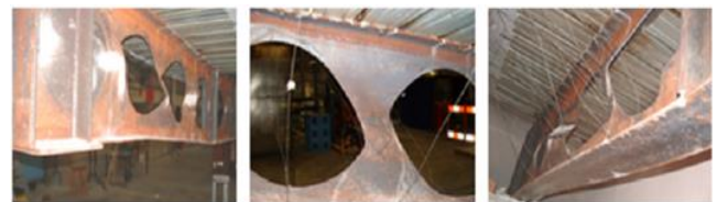
Figure 3 Web-post buckling failure at elevated temperature [29]
