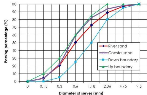
Figure 1 Gradation of river sand and coastal sand
