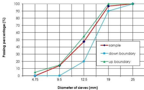
**Figure 2** Gradation of coastal aggregate
