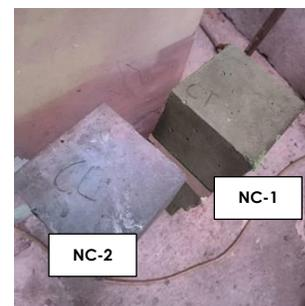
**Figure 6** Effect of curing on sampel surface
