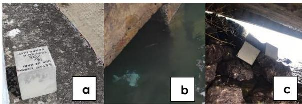
**Figure 4** Marine environment treatments: (a) CZT, (b) SZT, and (c) TZT
