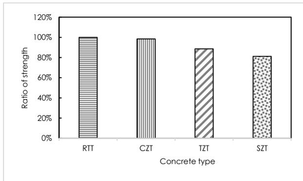
**Figure 10** Reduction of compressive strength due to environment effects
