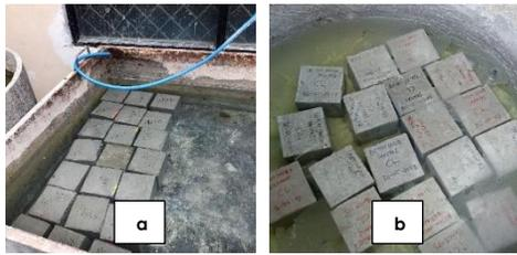
**Figure 3** Curing process: (a) in fresh water and (b) in seawater
