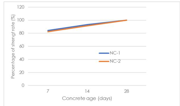
Figure 9 Rate of compressive strength due to curing condition
