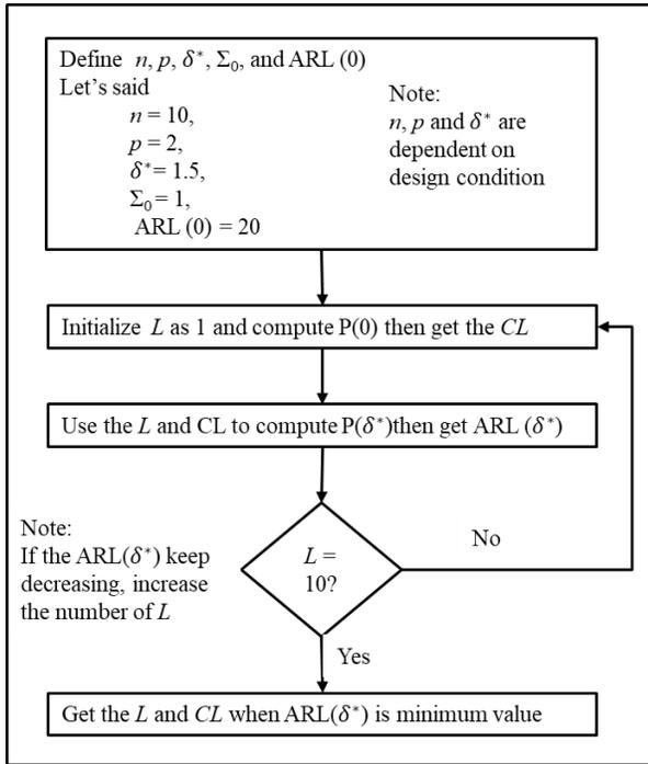
Figure 1 Flowchart to derive optimal parameters for robust control charts
