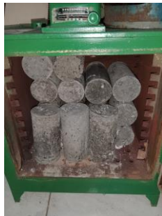
Figure 1 Curing process of geopolymer concrete using oven at 60°C for 4 hours
