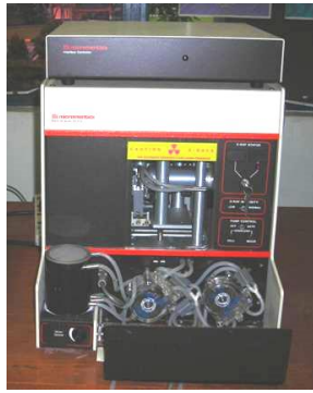
Picture 9 Analysing the mass size bunber using Micromatics 5100 Particle Size Analyser
