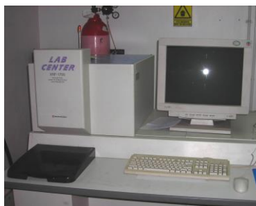
Picture 11 Analysing chemical composition using Shimadzu XRF-1700 X-ray Fluorescence Spectrometer
