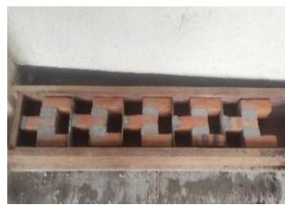
(b) The casting of shear specimens
