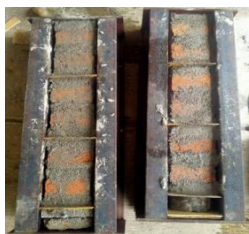
(a) The casting of brick pair sample
