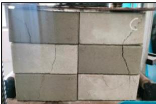
Figure 13a Failure of M0 prism
