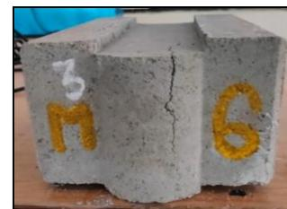
Figure 8g Failure of M6 brick
