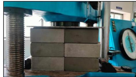
Figure 5 Test setup for prism
