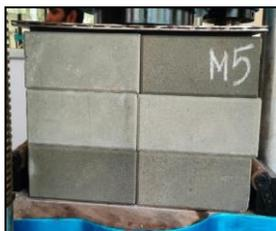
Figure 13f Failure of M5 prism
