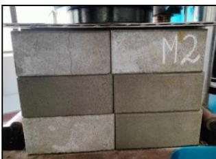
Figure 13c Failure of M2 prism
