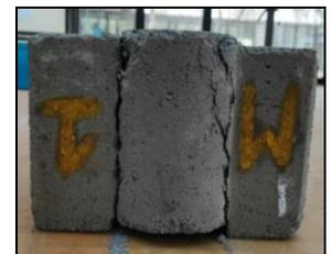
Figure 8b Failure of M1 brick
