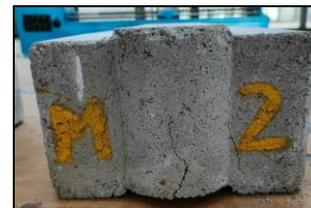
Figure 8c Failure of M2 brick
