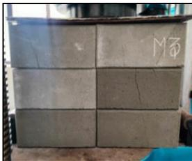
Figure 13d Failure of M3 prism
