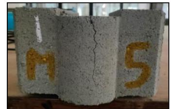
Figure 8f Failure of M5 brick
