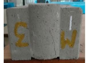
Figure 8d Failure of M3 brick
