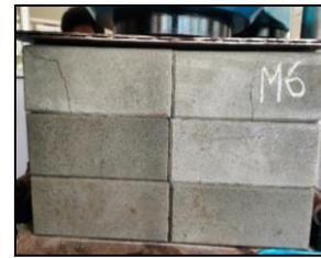
Figure 13g Failure of M6 prism
