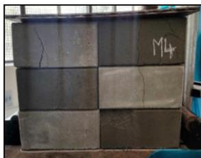
Figure 13e Failure of M4 prism
