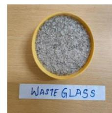
Figure. 1f. Waste glass after processing
