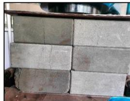
Figure 13b Failure of M1 prism
