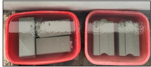
Figure 4 Water absorption test
