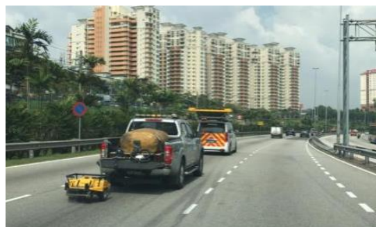
Figure 6 Mark 2 Grip Tester for Measuring Skid Resistance
