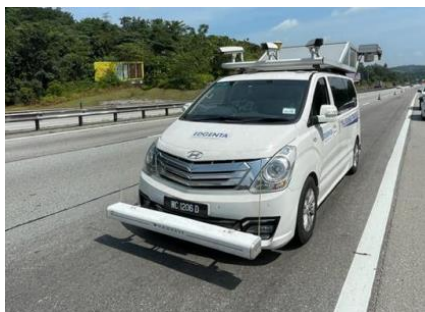
Figure 4 Scanning Road Surface by ARRB Hawkeye Survey Vehicle (Hawkeye 2000)
