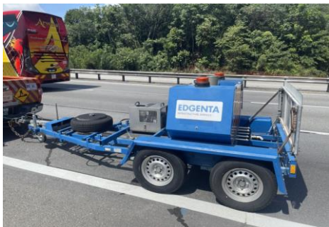
Figure 3 FWD Test in Progress
