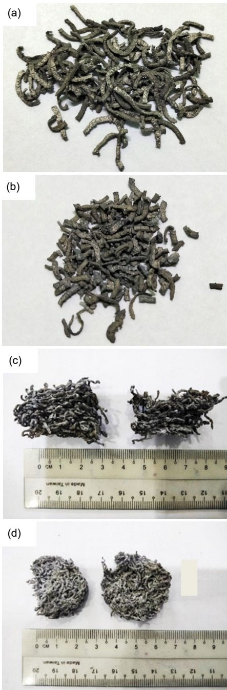
Figure 1 Heated aluminium chips (a) without flux at temperature 650°C; (b) without flux at temperature 700°C; (c) with flux at temperature 650°C; (d) with flux at temperature 700°C
