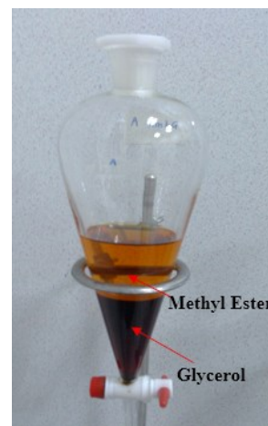
Figure 2 The base catalysed transesterification process of CJO to obtain JME
