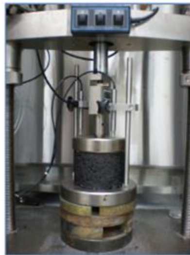
Figure 3 Fixing for creep test
