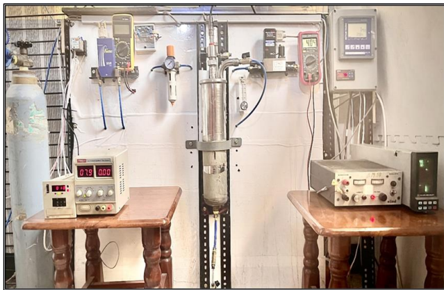
Figure 2(a) Photographic picture of apparatus used for semi-batch CO 2 absorption system
