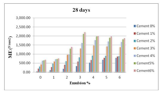
Figure 5 Effects of Cement - Bitumen Emulsion on ME (28 days)
