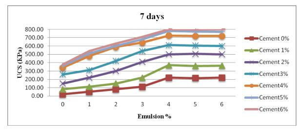
Figure 3 Effects of Cement - Bitumen Emulsion on UCS (7 days)
