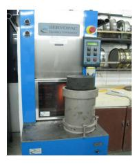
Figure 2 Superpave Gyratory Compactor (SGC)
