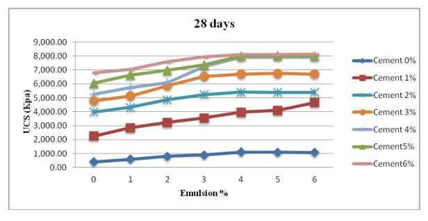
Figure 4 Effects of Cement - Bitumen Emulsion on UCS (28 days)
