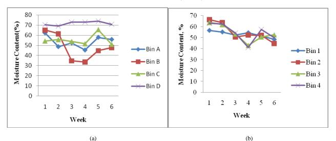
Figure 1 Moisture content by week in the composter barrel (a) and rotary drum (b)
