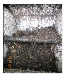
Figure 5 Compost products in rotary drum
