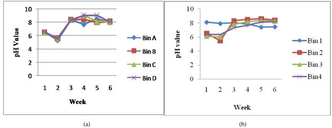
Figure 2 pH value by week in the composter barrel (a) and rotary drum (b)
