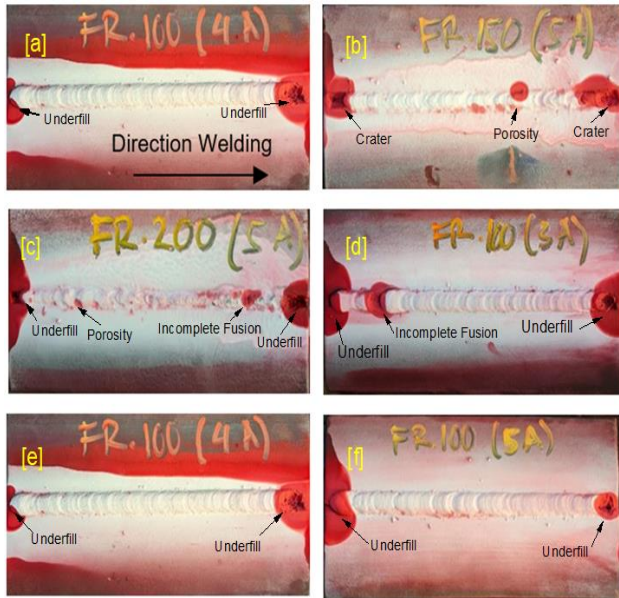
Figure 8 Results of welding and dye penetrant test, current parameters; (a) 70A,100 mm/min, (b) 80A,100 mm/min, (c) 90A,100 mm/min; Travel Speed Variation;(d) 80A,100 mm/min, (e) 80A,150 mm/min, and (d) 80A,200 mm/min
