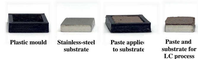
Figure 2 The plastic, stainless steel substrate and paste applied to stainless-steel surface
