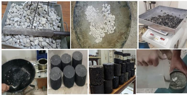
Figure 3 Preparation of Hot Mix Asphalt (HMA), Marshall Test Samples and Grouting
