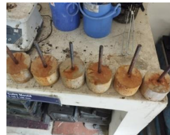
Figure 25 Test specimen after corrosion
