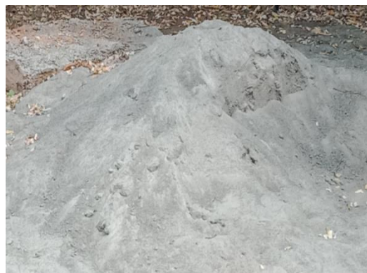
Figure 1 Manufactured Sand (MF-Sand)
