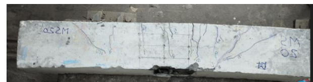
Figure 23b Crack Formation in the MR20 Beam
