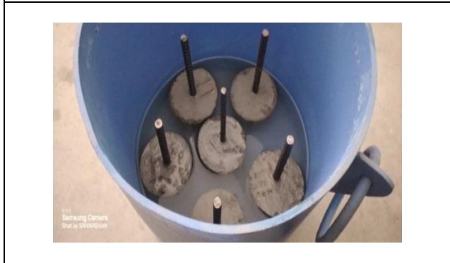
Figure 14 Curing of specimen for corrosion test
