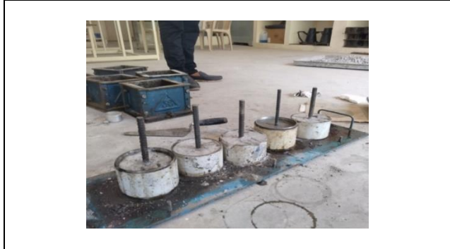
Figure 13 Casting of specimen for corrosion test
