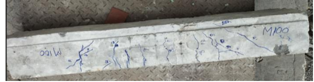
Figure 23a Crack Formation in the MF100 Beam
