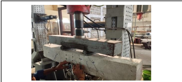
Figure 17 Measuring deflection and strain in the RCC beam
