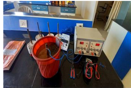
Figure 24 Corrosion Test Setup
