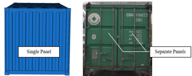
Figure 19 Door assembly of FEM (left) compared to the actual container (right).
