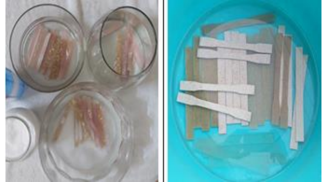
Figure 6 Immersing samples in acidic, basic, and water media
