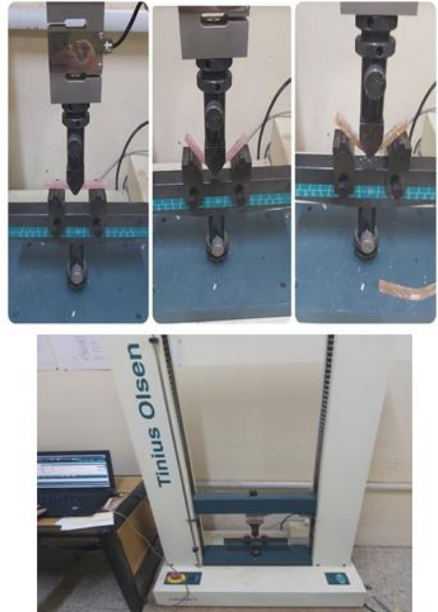
Figure 8 Three-point bending tests
