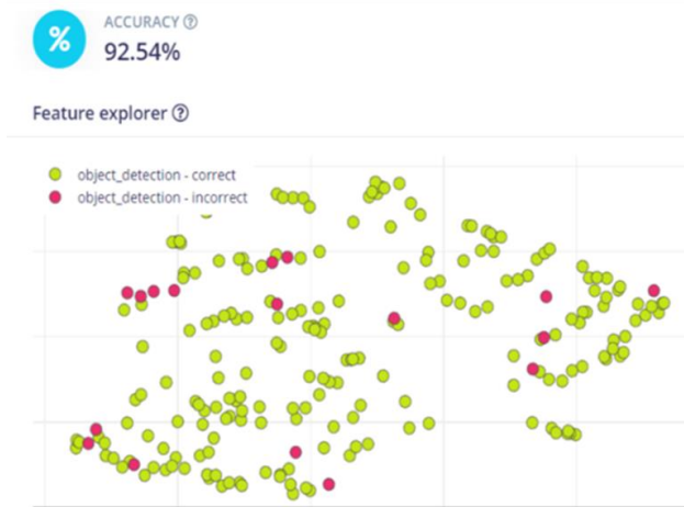
Figure 6 Accuracy and feature map of the FOMO model on the Arduino Nano BLE TinyML Kit, alpha value = 0.35, 140 epochs
