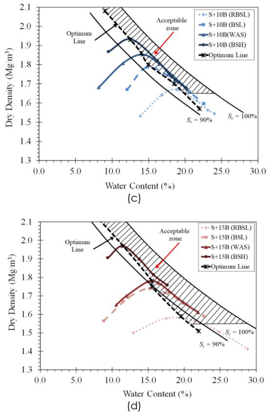
**Figure 4** Acceptance zone based on modern criterion for (a) Soil only (b) Soil+5B (c) Soil+10B and (d) Soil+15B
