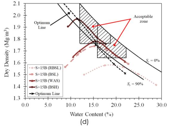
Figure 2 Acceptance zone based on traditional criterion for (a) Soil only (b) Soil+5B (c) Soil+10B and (d) Soil+15B
