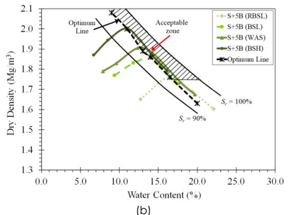
Figure 3 Acceptance zone based on common criterion for (a) Soil only (b) Soil+5B (c) Soil+10B and (d) Soil+15B
