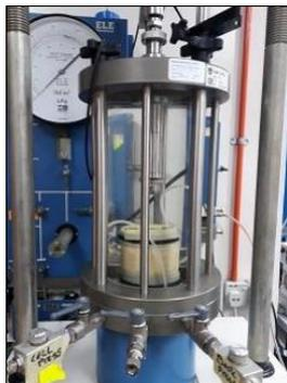
**Figure 1** Triaxial machine used for permeability testing to obtain hydraulic conductivity values
