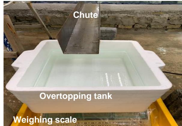
**Figure 5** Overtopping chute and overtopping tank placed on weighting scale to collect overtopping waves and measure overtopping volume
