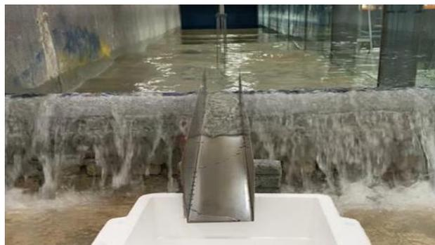
**Figure 11** The occurrence of the large individual wave overtopping during the experiment
