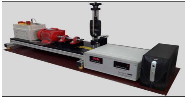
Figure 3 Machine of rotating bending fatigue test
