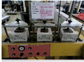
**Figure 4** Permeability test according to DIN EN 12390-8:2009-07
