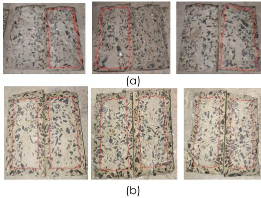
**Figure 10** Results of permeability testing using the split tensile method: (a) Permeability of submerged in seawater, (b) Permeability of submerged in brackish water
