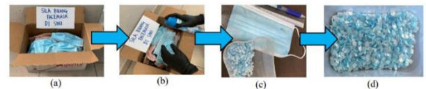
Figure 2 Disposable face masks (DFM) (a) collected in boxes, (b) disinfected with alcohol sanitizer liquid, (c) manually cut to 6 mm length strips, and (d) DFM strips
