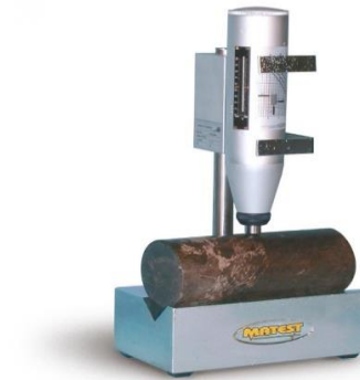
(f) Apparatus for measurement of laboratory Schmidt Rebound Hammer value, R
