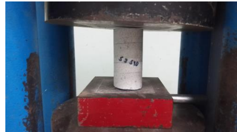
(e) Apparatus for measurement of uniaxial compressive strength, UCS
