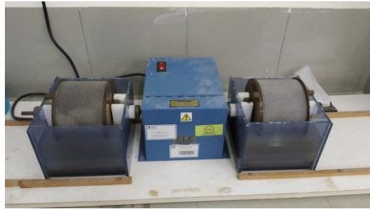
(b) Apparatus for measurement of slake durability index, Id 2
