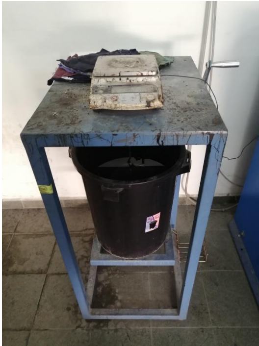
(a) Apparatus for measurement of specific gravity, porosity, and moisture content
