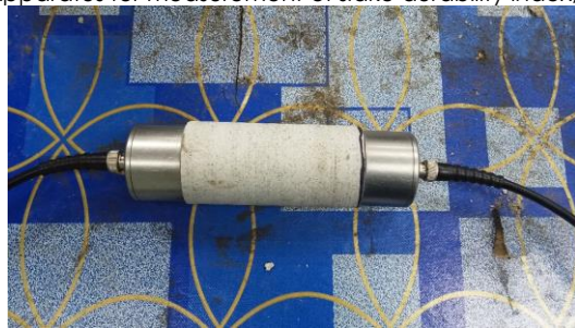
(c) Apparatus for measurement of ultrasonic pulse velocity, UPV
