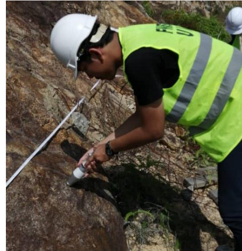
(b) Weathering grade measurement of slope using Schmidt Rebound Hammer
