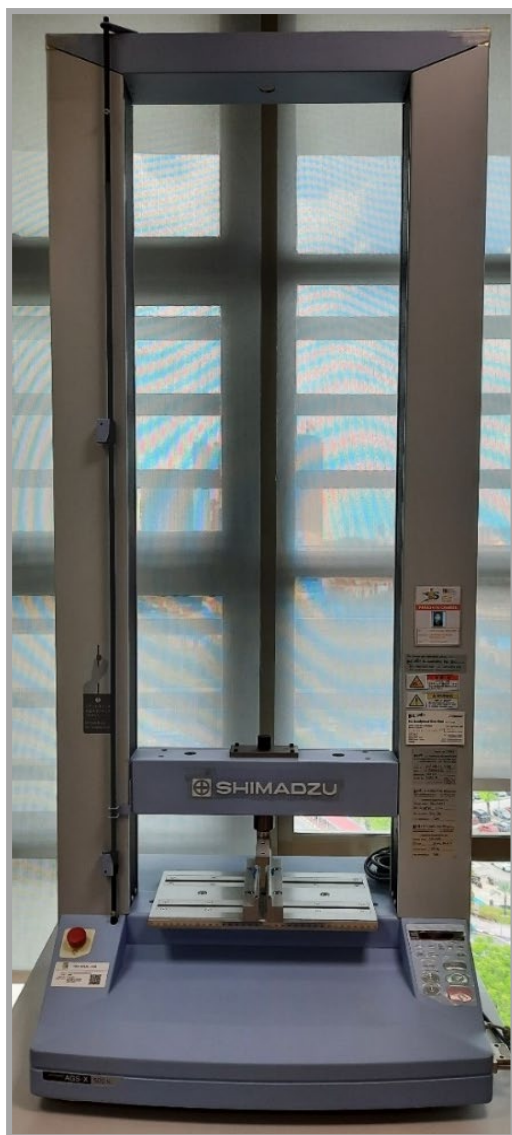
Figure 1 Instron Universal Test Machine (Shimadzu AG-X 500N Series)
