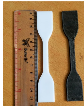
Figure 9 ASTM D638 Type IV commercial PLA (left) and rPLA specimens (right)
