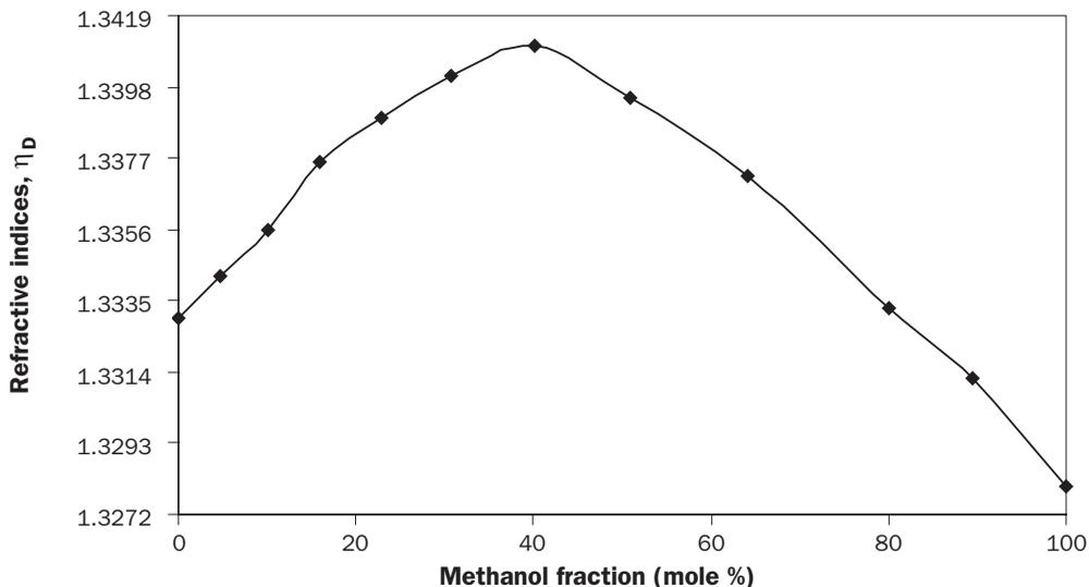
**Figure 1** Refractive index of methanol-water mixtures against mole fraction of methanol
