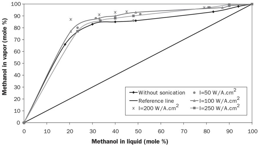
**Figure 3** Equilibrium curve of methanol-water system with different ultrasonic intensity at frequency of 40 kHz
