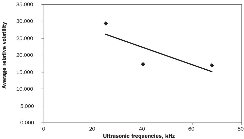
**Figure 6** Relative volatility of methanol-water system with different ultrasonic frequency at intensity 200 W/A.cm<sup>2</sup>
