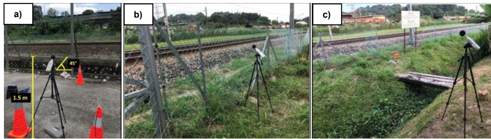
Figure 5 (a) SLM setup (b) SLM at D1 (c) SLM at D2 near residential area
