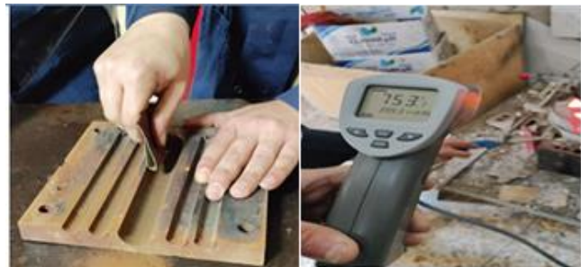
Figure 7 Cleaning and heating the mold
