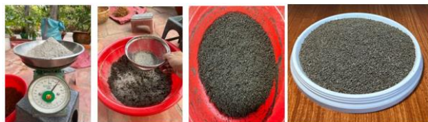
Figure 2 Cocopeat after being “hardened” with cement
