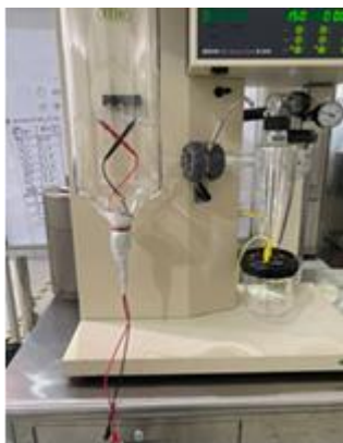
Figure 2 Preparation setup for the charges profiling of spray drying
