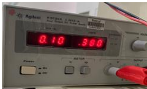
Figure 1 Dual output DC power supply for supplying electroconductivity charges prior to profiling measurement
