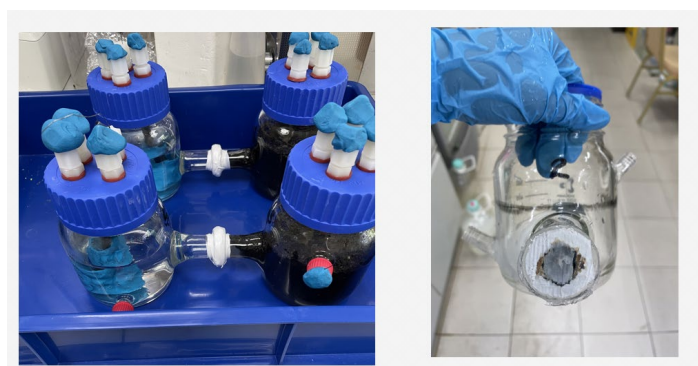
Figure 12 Example illustration of application of the ion exchange membrane in microbial fuel cell-based dewatered sludge
