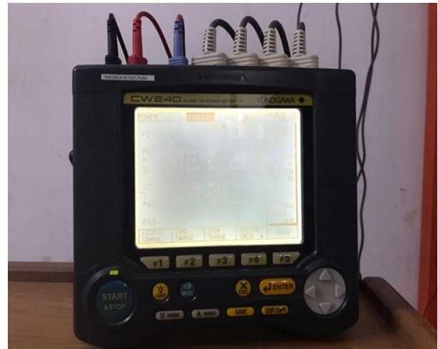
Figure 16 Power Analyser to measure energy consumption
