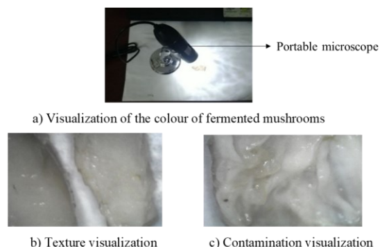
Figure 3 Quality control visualization and assessment of the fermented mushrooms via: a) colour; b) textural & c) contamination and fungal growth
