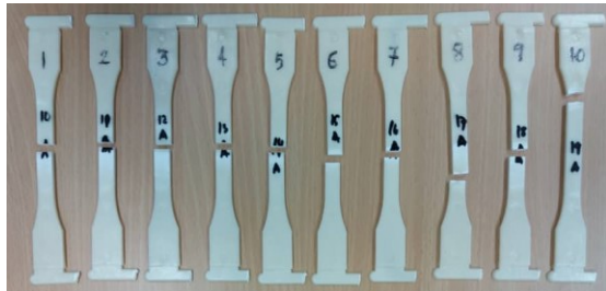
Figure 19 Tensile strength specimen failure area for MEC molded part
