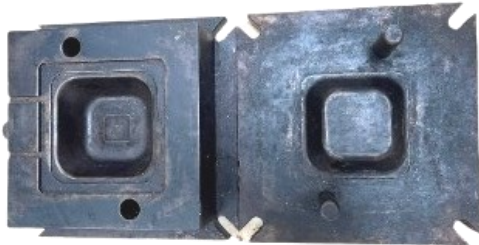
Figure 1 Carbon steel mold system used in the forming process
